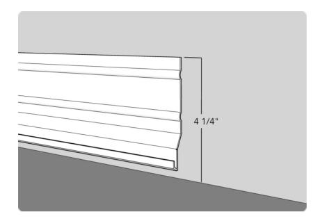
2. Screw the starter strip into place. Place screws every 8 inches to minimize movement of the starter strip. Leave ½" in between each starter strip to allow for expansion/contraction. Apply a building cladding tape over the top of the starter strip.
