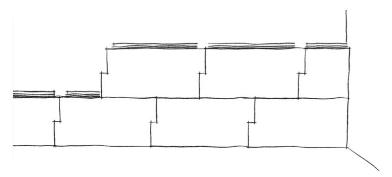
10. As each course is installed, ensure the flange of each panel has been installed in the groove of the panel below and the vertical edges are in contact with the adjacent panel.
